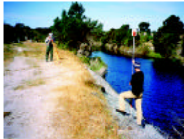
Surveying of drains for the model of how the drains work to assist with improved drain management
